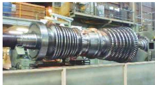
Shroud machining of HIP rotor at MHI-Nagasaki for 800 MW turbine for Andhra Pradesh Power Development Company
